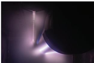
Gencoa's active anode provides an effective method for collecting electrons escaping rotatable magnetron plasma (low impedance plasma patent 9028660, filed August 14, 2008).
